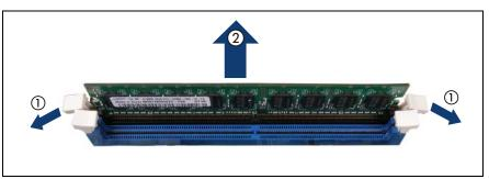
Figure 35: Removing a memory module
